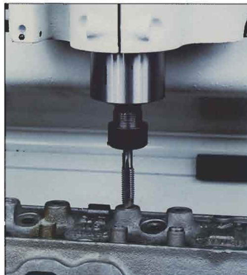
Drilling and tapping for screw-in studs and removal of broken exhaust studs is easy with the VGS-20.
