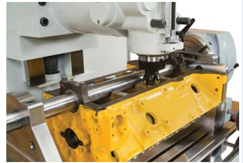
RMC's Shell Mill Tooling allows use of RMC's shell mill option to perform a variety of regular machining operations
