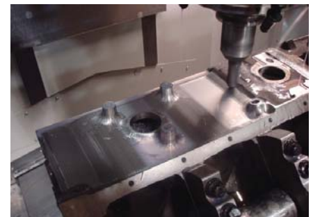
RMC's Block Lightening Tooling Package
