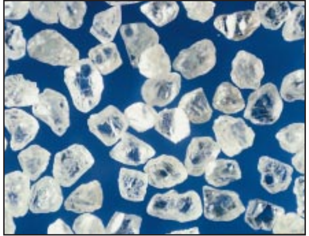
Sunnen diamond abrasives (as shown in magnified photo above) are essential in the honing of glass, quartz, tungsten carbide and ceramics. Photo courtesy of Diamond Abrasive Corporation.
